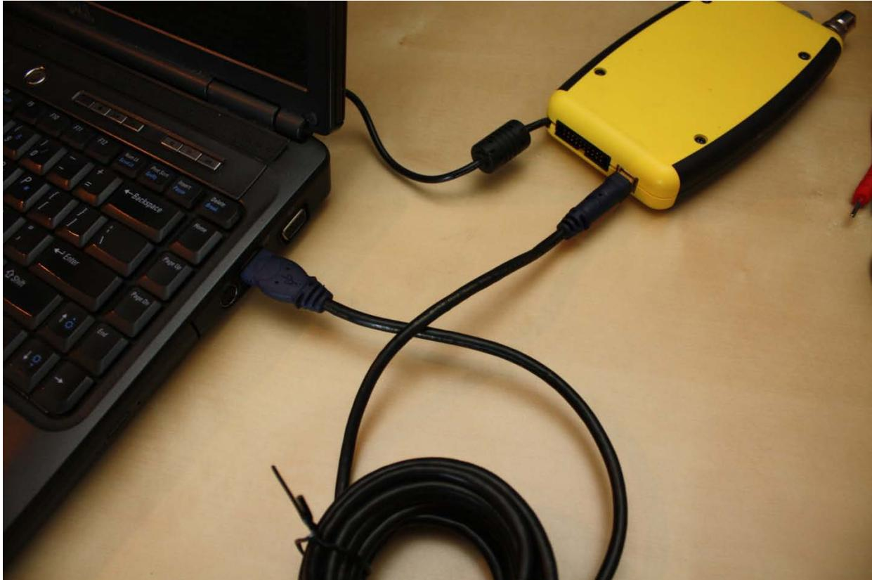
Now, once you have the USB cable connected, the green LED light will turn on. If the green light doesn't come on, then there is a problem either with the cable, device or computer/Windows.
