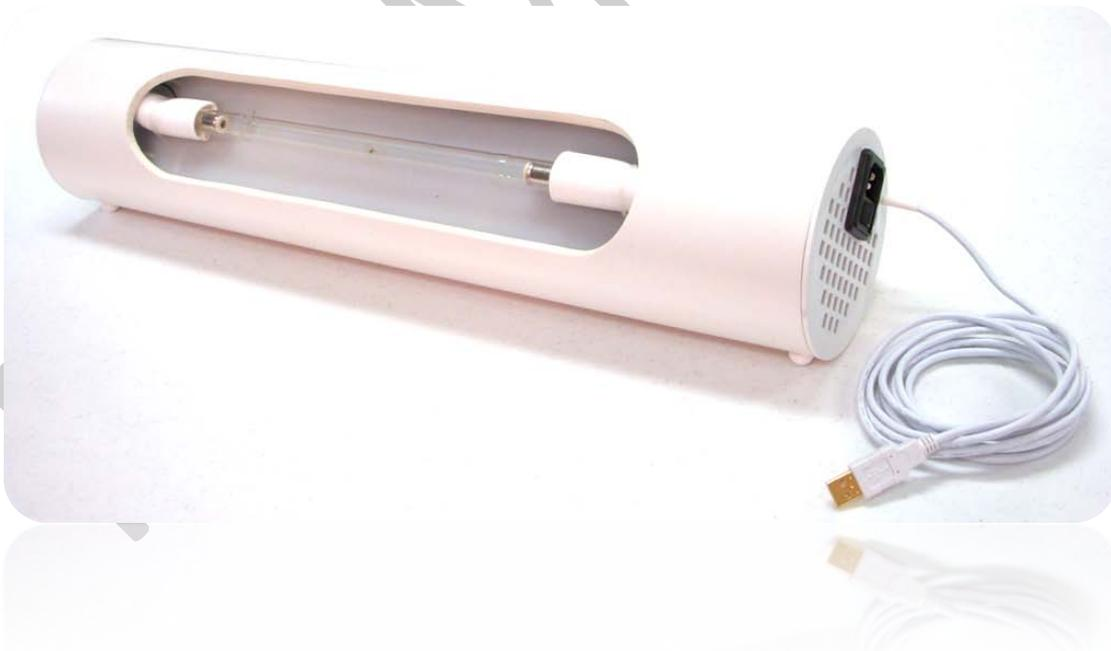
In this picture: a P3+ unit. Notice, there's only one USB cable, a connector for the power cord and a power switch. Both standard and custom configurations may vary slightly.
